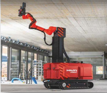
Automated Drilling Robot
