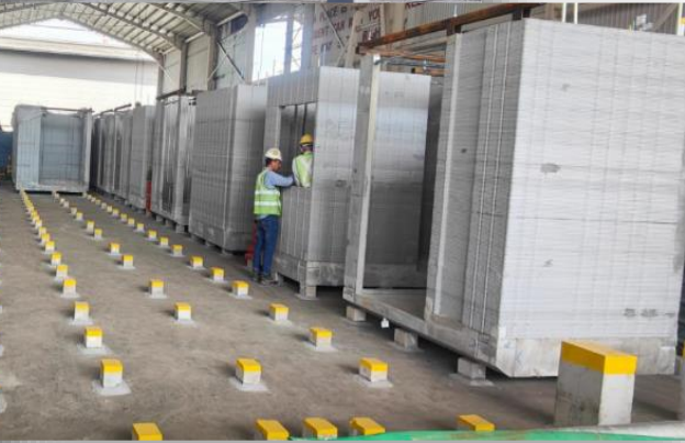
3D Concrete Printed PBUs
