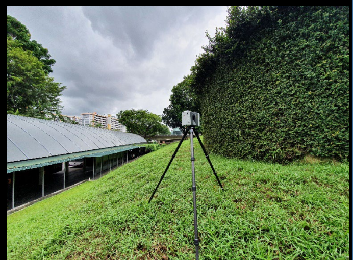
Leica 3D laser scan for BIM Model creation of Existing Station
