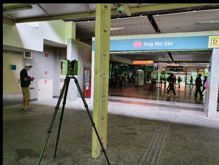
Leica 3D laser scan for BIM Model creation of Existing Station
