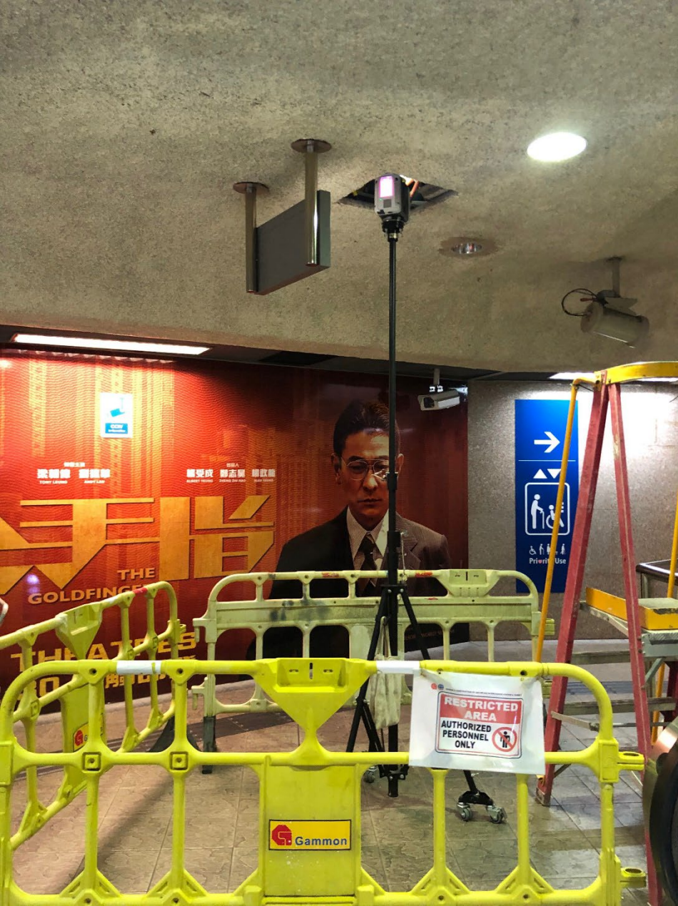
Leica 3D laser scan for BIM Model creation of Existing Station
