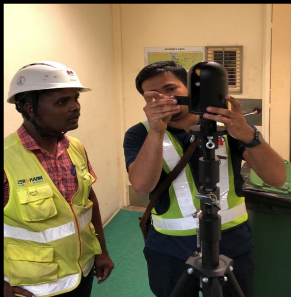
Leica 3D laser scan for BIM Model creation of Existing Station
