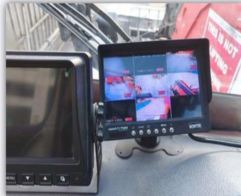
In-cabin monitor screen provided for operator
